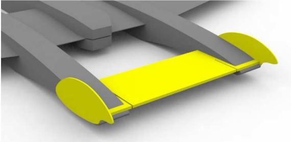
**Step10** If you are making the Warlock in a pusher configuration attach the motor mount to the rear of the fuselage.
