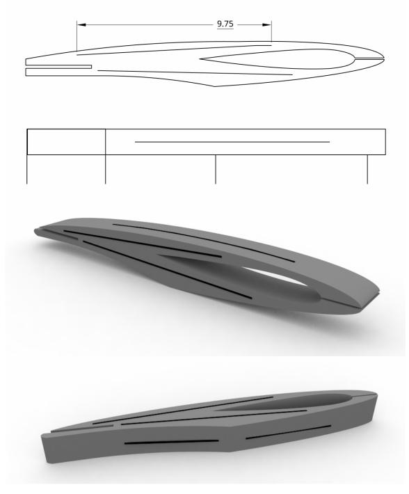
Cut and add the spars to your wing. Be careful that you make sure the wing is straight and without warp as the glue dries. Pay particular attention to the outer wing panels as they are tapered. Be sure to spar top and bottom of the wing.
