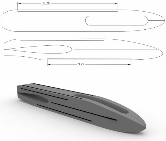
**Boom Spars** Cut the boom spars to 9.75" length and install them on the top, bottom and sides of the booms as shown.
