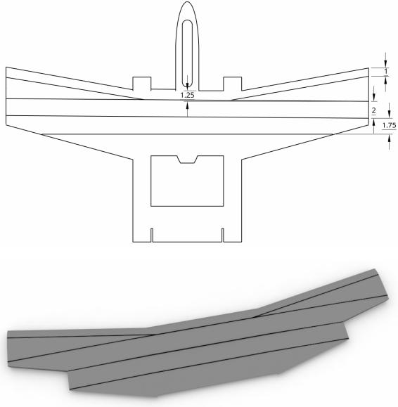
Laminate the wing with the supplied laminate. Cut out spaces in the laminate for where the booms and fuselage will attach. This way when we attach them they will be glued foam to foam for the best bond possible.
