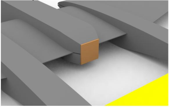
Cut the fuselage battery plug to the desired height and glue it in place inside the fuselage.
