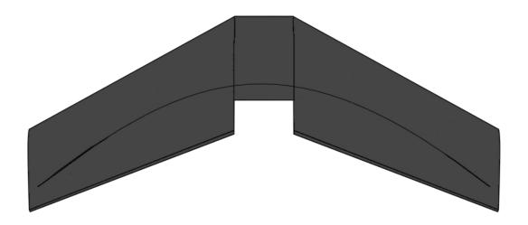
On the underside of your wing lay the short spar across the nose and bend the ends down. Mark this line and cut and glue the spar in place like you did in the previous step for the long spar
