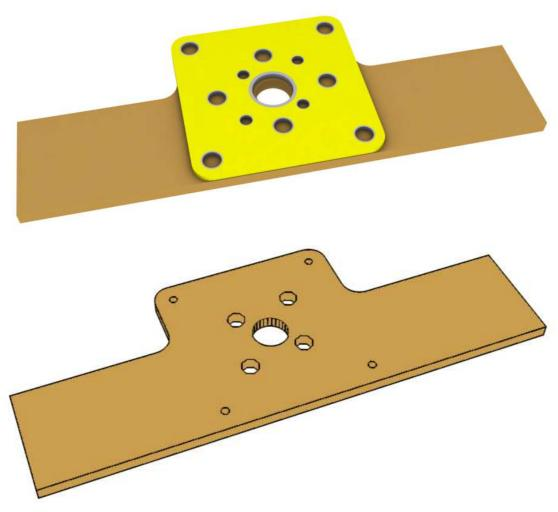
**Step11** Glue the motor mount to the rear of the aeroplane
