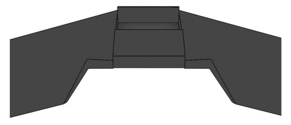
These foam fins are an option addition to the Apex. Glue the foam fins to the side of the blunt section.
