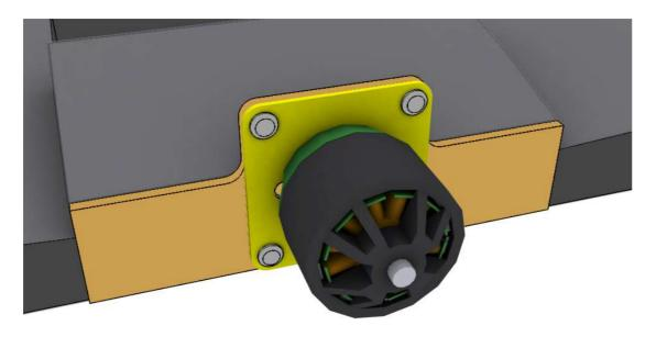
Cut holes for your servos on the top of your wing where you want them to be installed. We strongly recommend you do this in front of or on the CG line as this will help balancing your plane later on.
