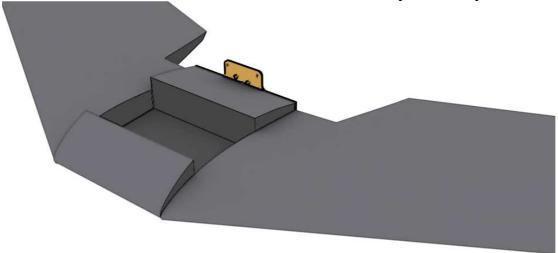
Laminate your elevons. Cut in and glue in the control horns on your elevons, install them in such a way that the holes are directly over the edge where the elevon will meet the wing. Cut 4 strips of laminate the length of your elevons and about 2 inches wide. Using these as top and bottom hinges, use your hobby iron to attach the elevons to the wing.
