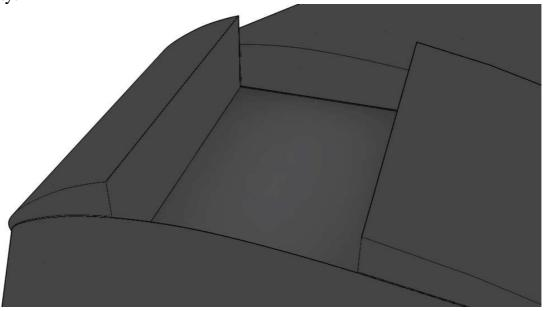
**Step7**Identify how big of a propeller you're wanting to use on your build and cut out the back corner of the wings to ensure you have enough clearance.
